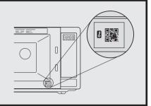
6. If the Wi-Fi icon stops blinking and is off after 5 minutes, reset the microwave oven by pressing Wi-Fi CONNECT button restart from the step 5.
