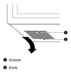
**2** Soak grease filters in hot water and a mild detergent.
