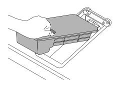
2 Hold the filter assembly over a trash can and pull the handle on the front of the filter to slide the mesh filter off as shown.
