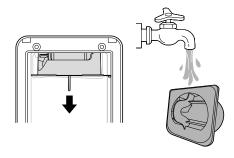
Clean the inside thoroughly with a nylon brush (not provided). Do not touch the condenser fins with bare hands. After cleaning, reassemble the protective grille and insert and tighten the screw.
