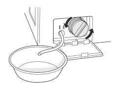
Clean the pump filter and opening.
