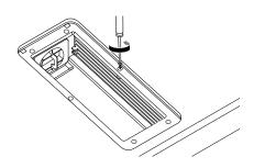
Tilt the protective grille for the condenser slightly to the left and pull it out to remove.
