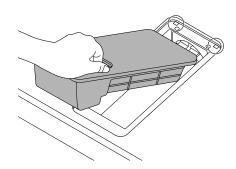
LG recommends periodic cleaning of the condenser area for thorough cleaning. To clean, loosen the screw with a Phillips screwdriver.
