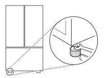
2 Open both doors and check to make sure that they close easily. If the doors do not close easily, tilt the refrigerator slightly more to the rear by turning both leveling legs to the left. It may take several more turns, and be sure to turn both leveling legs the same amount.
