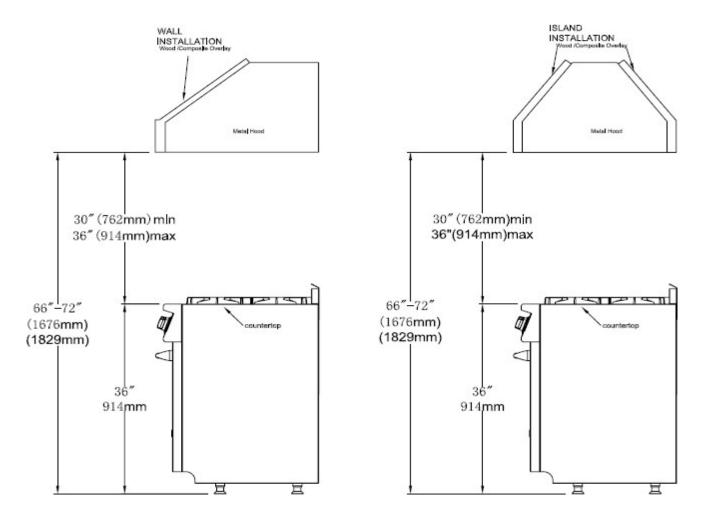
The bottom of the hood should be 30" min. to 36" above the counter top. This would typically result in the bottom of the hood being 66" to 72" above the floor. These dimensions provide safe and efficient operation of the hood.
