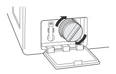
Close the drain pump filter cover.
